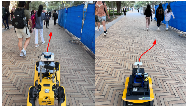
Fig. 1: A human demonstrator teleoperates the two robots, following a socially compliant strategy (left- moving with traffic, right- sticking to the right of the road) around human crowds.
