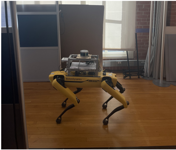
Fig. 2: The Boston Dynamics Spot robot as equipped for this study; including a laptop, Velodyne VLP-16 LiDAR, and a Microsoft Azure Kinect point cloud camera.
